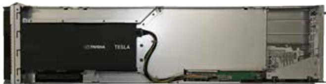
Picture 4. V205F double-width CM with NVIDIA Tesla M2090 accelerator (top view, w/o duct cover)
