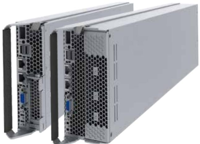
Picture 5. V205S (left) and V205F (right) compute modules
