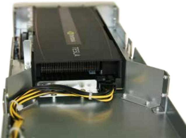
Picture 7. V205F CM with NVIDIA Tesla M2090 accelerator
